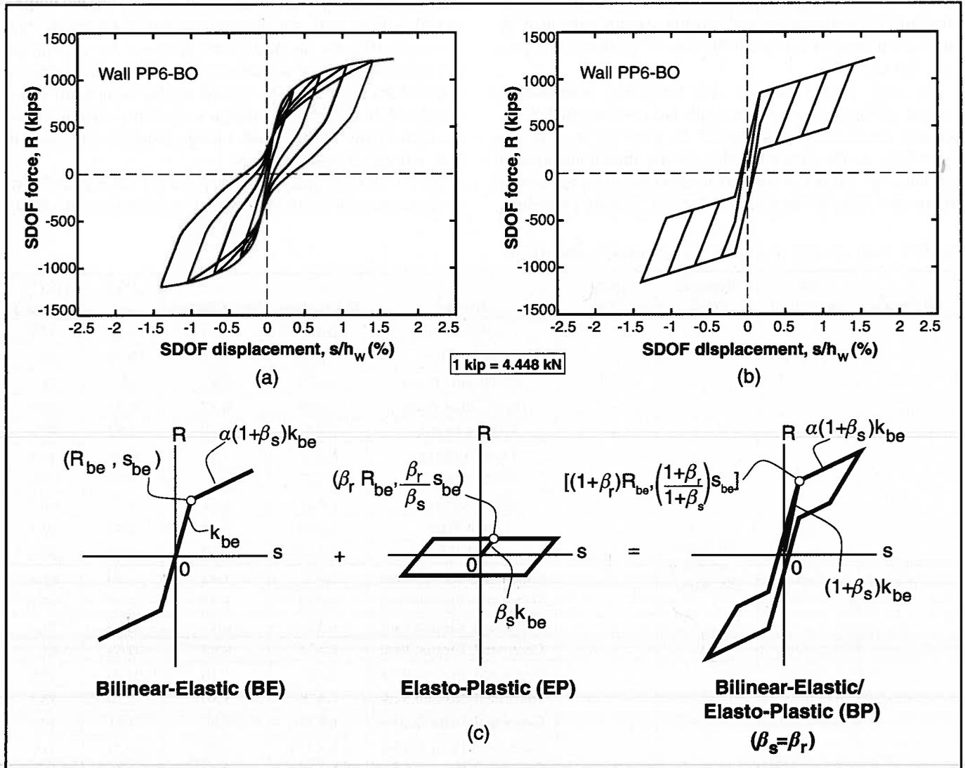
Fig. 8. Equivalent single-degree-of-freedom force-displacement ( $R-s$ ) relationship: (a) smooth  $R-s$  relationship; (b) idealized BP system  $R-s$  relationship; (c) components of BP system.
