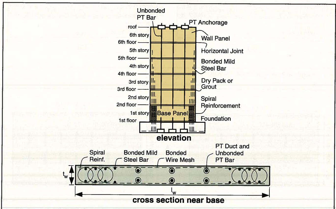
Fig. 1. Partially post-tensioned precast concrete wall.
