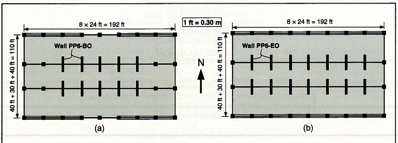
Fig. 3. Plan view of prototype buildings: (a) Building PP6-BO; (b) Building PP6-EO.
