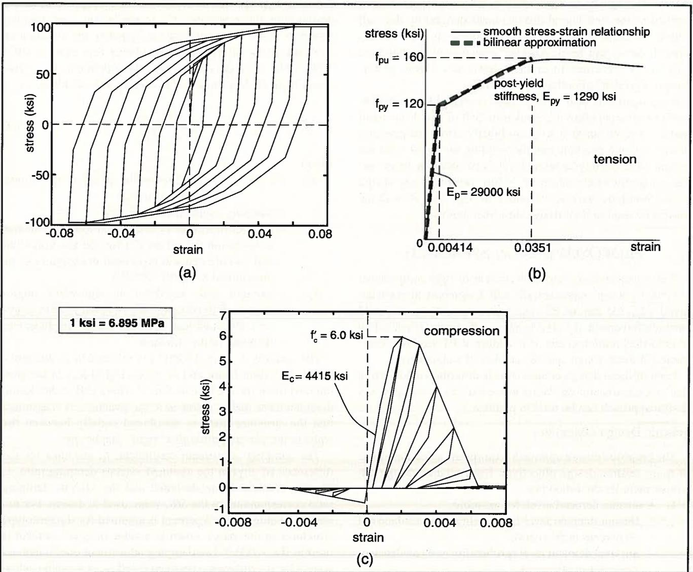
Fig. 4. Design/analysis material properties: (a) mild reinforcing steel; (b) post-tensioning steel; (c) unconfined concrete.
