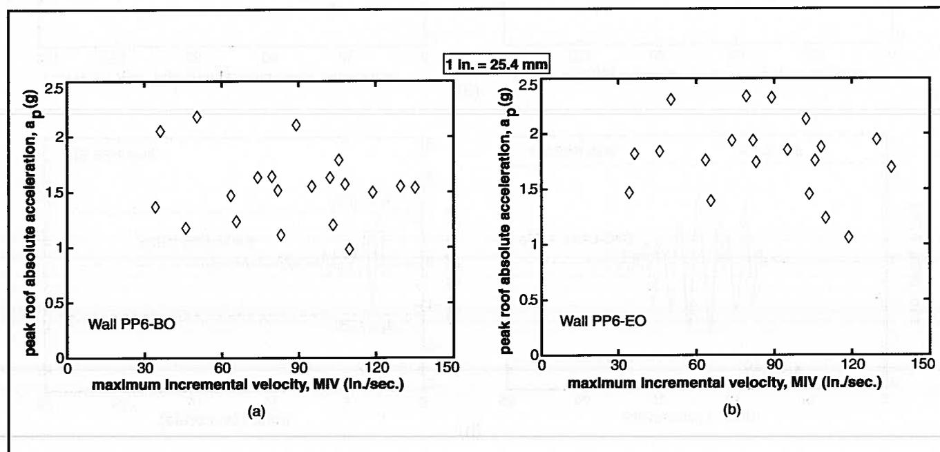
Fig. 11. Peak roof absolute acceleration of the prototype walls: (a) Wall PP6-BO; (b) Wall PP6-EO.
