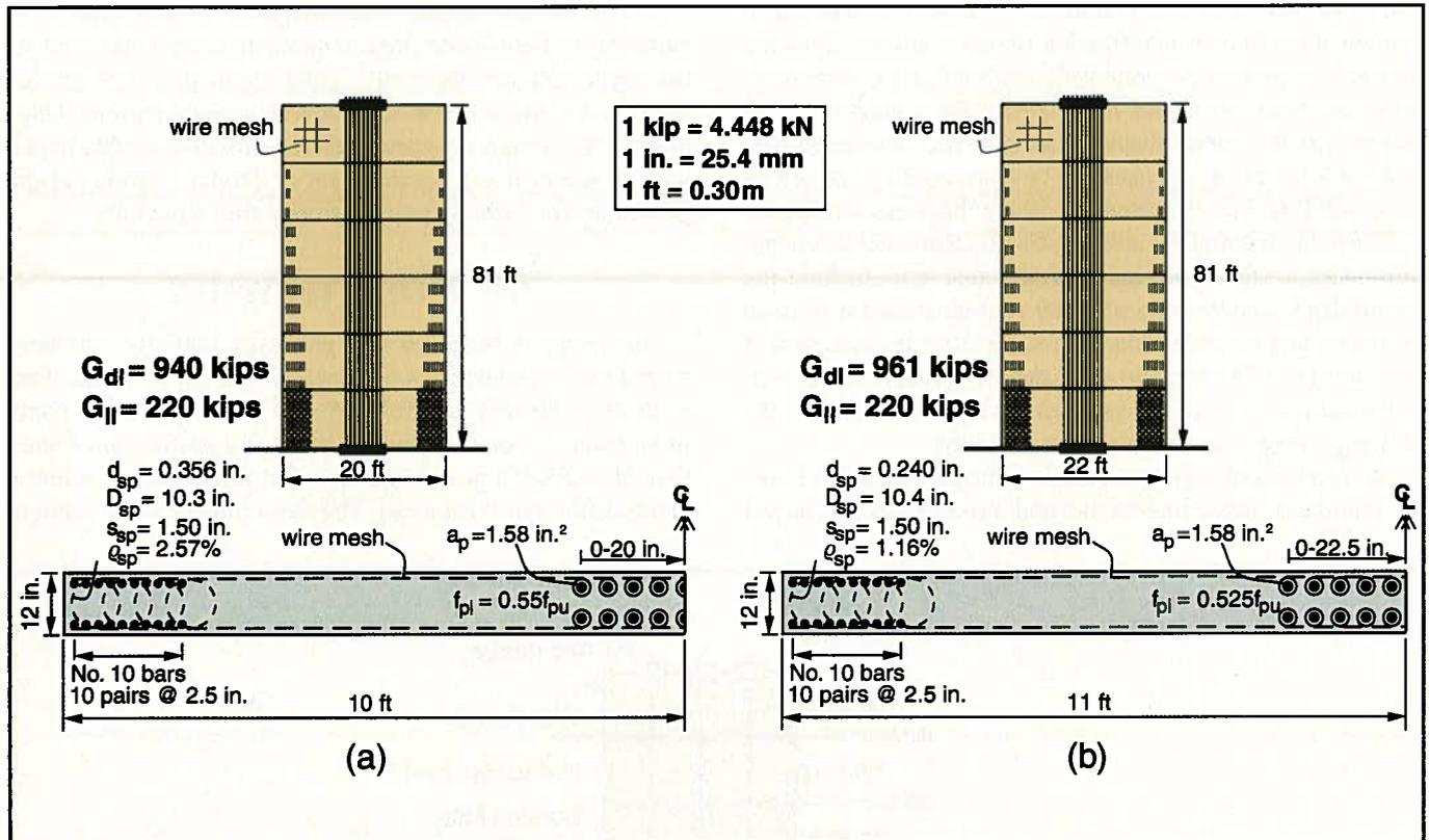
Fig. 2. Prototype walls: (a) Wall PP6-BO; (b) Wall PP6-EO.
