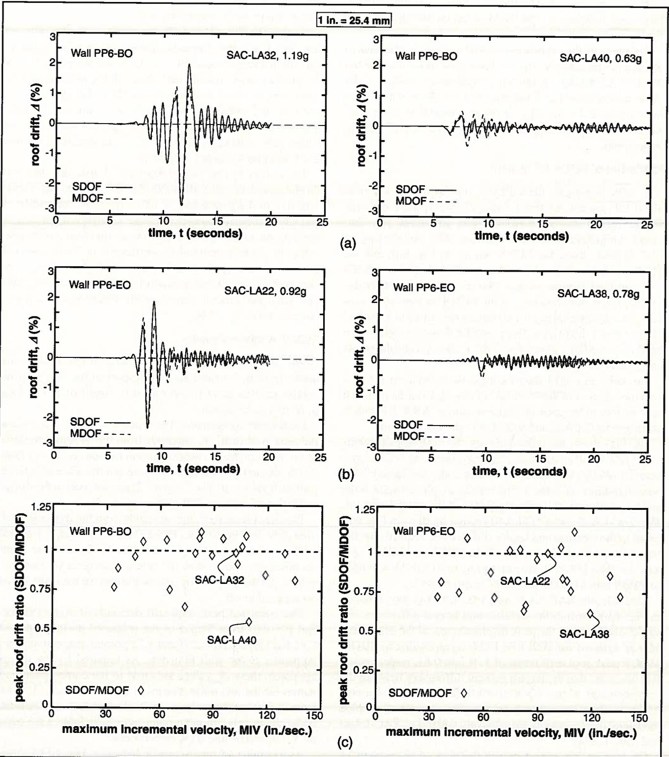
Fig. 9. Single-degree-of-freedom representation of the prototype walls: (a) roof drift time-history, Wall PP6-BO; (b) roof drift time-history, Wall PP6-EO; (c) peak roof drift ratio (SDOF/MDOF).
